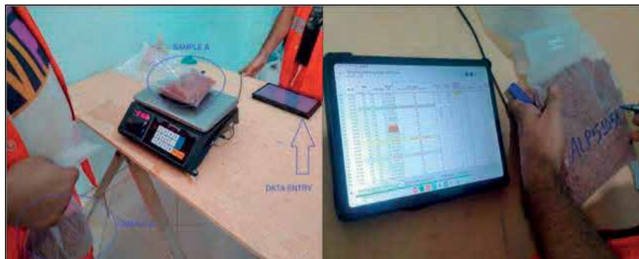
Figure 37: Samples being weighed for use as laboratory samples (left); Data base entry management on tablet for auger sample entry(right). Source: CSA Global 2023
