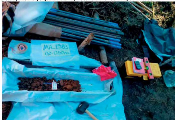
Figure 3. Sample collection after removal from auger bit. Bit cleaned with wire brush, while samples are removed using rubber hammer.
