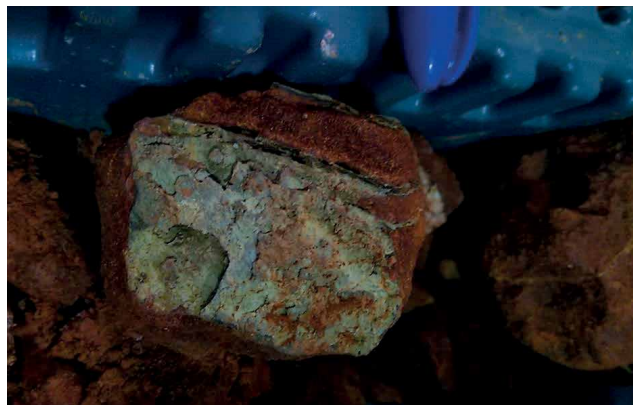
Figure 16. Secondary monazite coating fracture of friable monazite rich saprolite.
