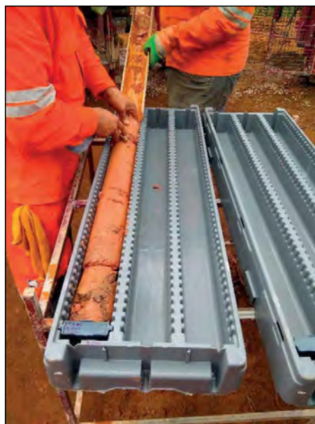
Figure 33: Clay regolith boxed into 10cm graduated plastic core boxes Source : CSA Global 2023
