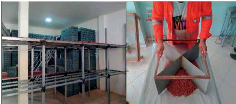
Figure 36: Sonic drill core storage Galpao (left); Cone and quartering of 1 m auger sample (right). Source: CSA Global 2023
