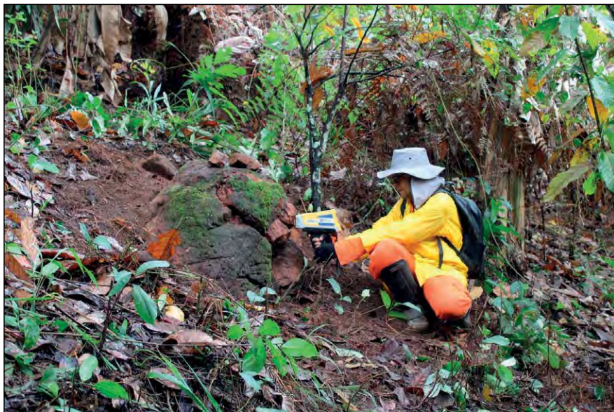
Figure 10. Example of subcrop being tested by pXRF (ALP400028 – 0.51 kg at 405000 ppm (40.5%) TREO (5% HREO and 20% MREO & 7% NdPr) Source: BRE 2023
