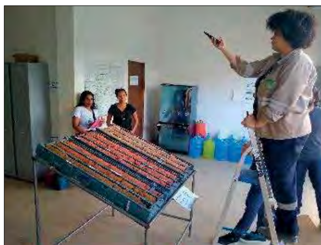
Figure 9. Core photography being carried out.
