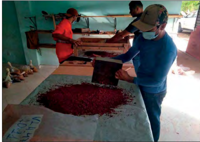
Figure 11. Drying, sieving and homogenisation of single 1-meter auger samples.
