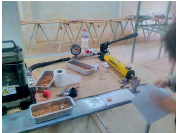
Figure 10. Vacuum apparatus and preparation of compressed clay discs for XRF analysis. The pellet may be noted on the sheet of paper and is the correct size for use in the hands free XRF unit used.
