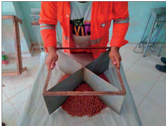
Figure 12. Cone and quartering of 1 m auger sample.
