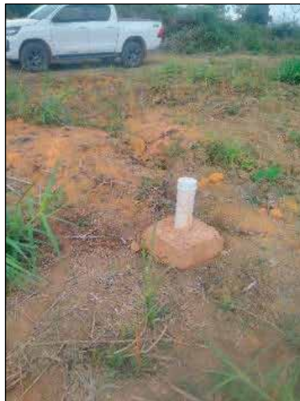
Figure 35: Drill collar for sonic drill hole in the field Source: CSA Global 2023
